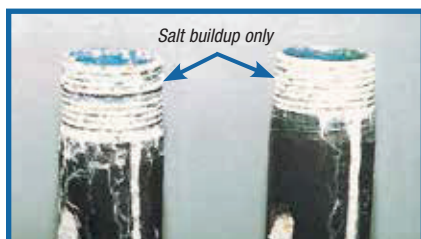
Example of Hot-Dip Galvanized Threads after 42-day salt-fog test
